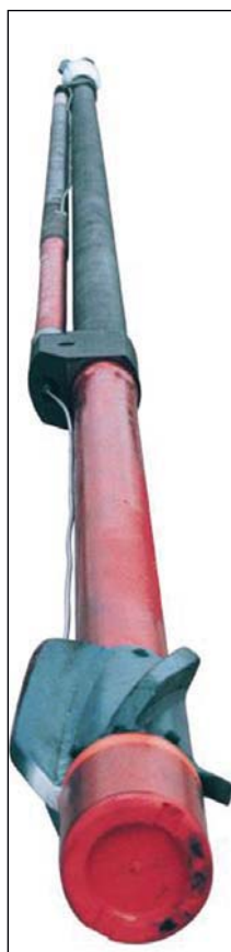
The Cana 1-15H well had 10 casing-conveyed perforating modules run in the well (Fig. 4). Photo from Marathon.
