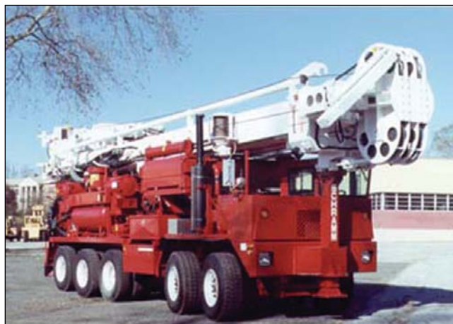
Major Drilling uses 760-hp Schramm T130XD Rotadrill carrier-mounted drilling rigs with telescoping masts to drill for CBM in the US (Fig. 3; photo from Major Drilling).
